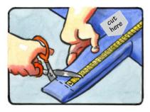
Mark half of the just measured length and shorten the tubular elements accordingly
